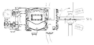
8. Check the valve stroke. The stroke marks are indicated on the feedback lever of the positioner. Position the connection pin at the number on the feedback lever which corresponds to the desired valve stroke. To adjust, move the bracket, the connection pin or both.
