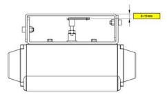
6. Attach the positioner to the bracket. Fix the clamping pin on the main shaft's center of the positioner and insert connection pin into the fork lever slot. This will lock to the fork lever spring. Setting alignment of the main shaft of the positioner and center of the actuator's stem is very important. Poor alignment of the main shaft and the actuator's stem decreases the positioner's durability due to unnecessary forces on the main shaft.
