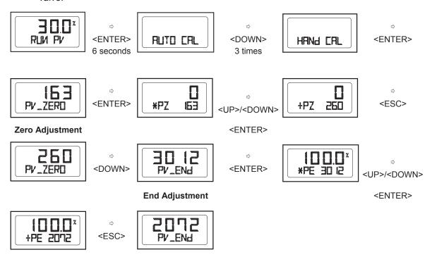
6.3.4.2 Zero-Point (TR\_ZERO) and End-Point (TR\_END) for Transmitter TR\_ZERO adjusts the zero point of the transmitter (4-20mA feedback), and TR END adjusts the end point of the transmitter (4-20mA feedback)
