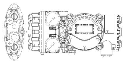
Fig. 10: Variable orifice adjustment
