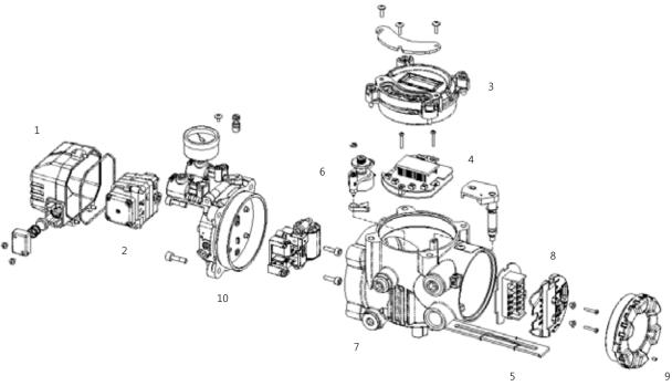
Fig. 2: YT-3400/3450 series exploded view
