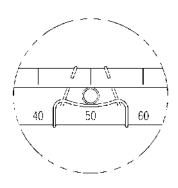
Proper way to connect feedback lever, connection pin, and lever spring
